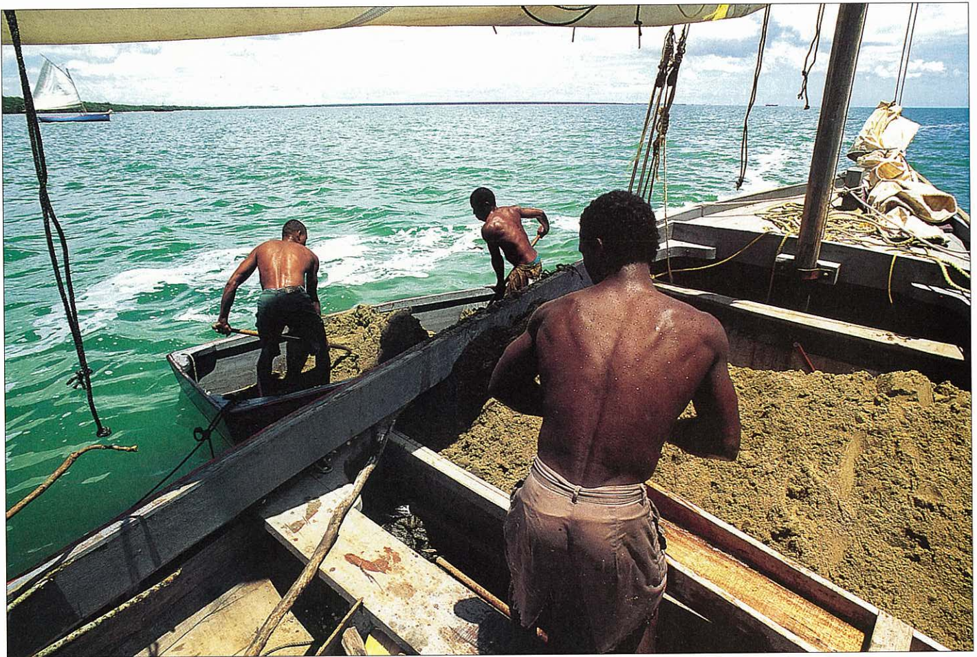
Loading a sand lighter: one member of the crew works the simple bilge pump while the others shovel sand from the skiff to the hold.
