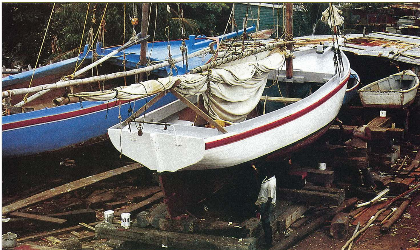
The Jones Boat Yard in Belize City can easily accommodate several boats at a time during their pre-regatta overhaul. Its wooden slipways are big enough to take two lighters at once. To aid windward performance, some of these half-decked boats are fitted with a false keel just for the racing!
